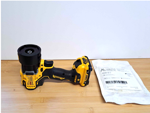
1 - Lay drill on back, peel open SteriGo
