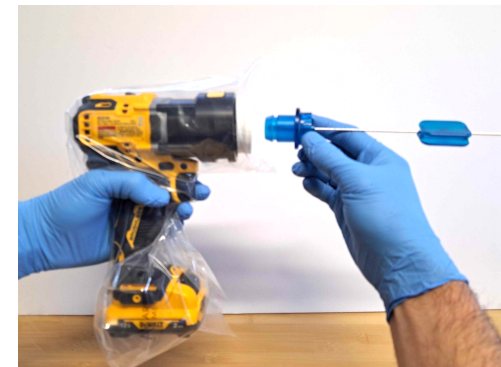
9 - Insert SteriTrak pin into drill until it clicks
